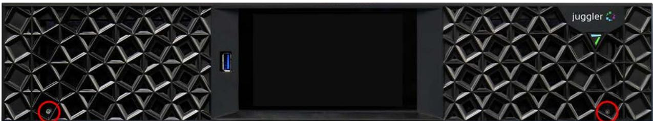
Remove the two small retaining screws bottom left and right, and then pull the fascia off its push-fit fasteners. Refit the fascia after mounting. Where side access is restricted for unranking, a 7thSense tool is available to insert into the grille. Take care not to damage the grille with other tools, or force when removing.
