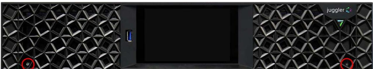
The front fascia can then be pulled straight off. The right-side filter has a cutout for the power switch. Each filter pad is simply fitted under the respective rails.
