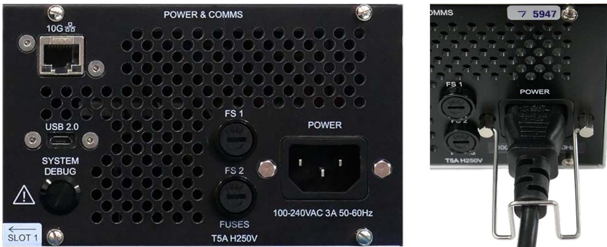
To the left of this are the two fuses for each internal power supply. (For replacement, see [Care and Maintenance](#) <sup>9</sup>.)
