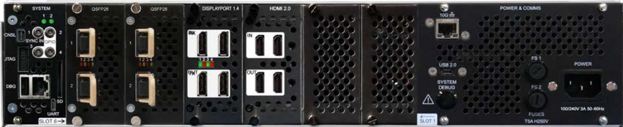
The I/O cards in slots 6-1 (numbered right to left) are push-fit but are not hot-swappable. The firmware of each Juggler 2 unit is custom to the physical arrangement of the unit. The example above shows two QSFP 28 cards, which can be used for optical bus or ST 2110 functionality, one HDMI 2.0 card and one DisplayPort 1.4.
