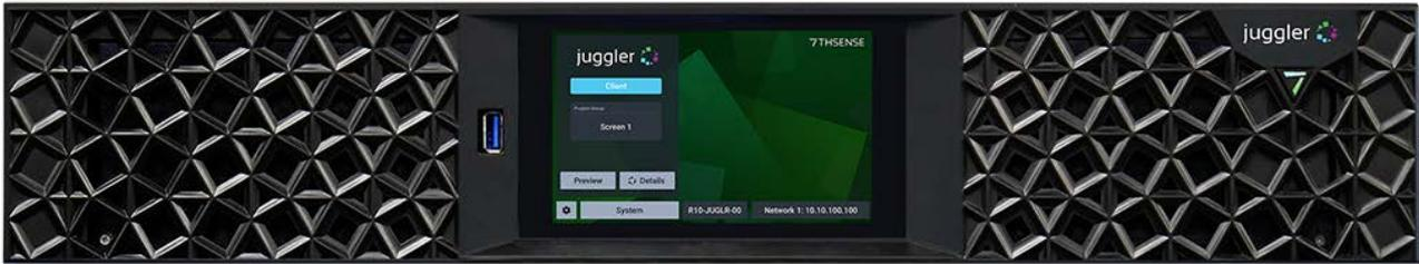
The Juggler 2 front panel has a touch-screen display, the 7-symbol power button (recessed into the fascia, top right) and a single USB 3 connector to the internal processor that runs Compere and the front panel display. The USB connector is for keyboard access to the internal processor (single board computer running Linux).
